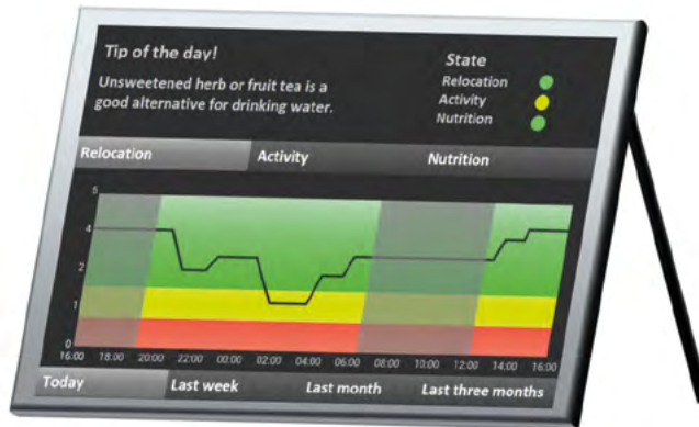
Figure 2 Visualization of sensor data on the tablet. The number of 15 min intervals with at least one re-positioning within 60 min is plotted over time.
