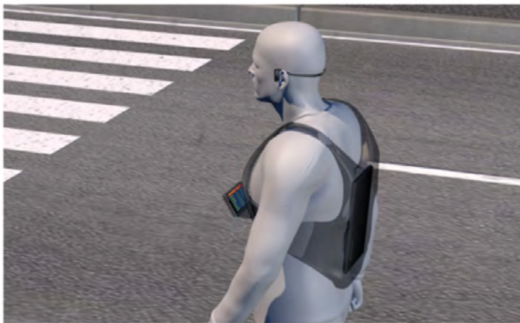
Figure 1 Alice device consists of smartphone wirelessly connected to a remote processing unit.
